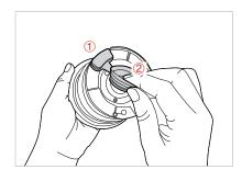
The silicone cover is removable for cleaning. After cleaning, place the silicone cover in regular sequence on as shown in the picture.
