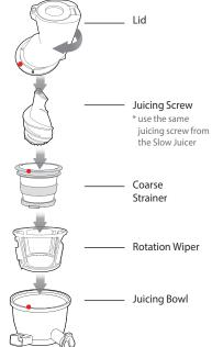
\* When using the coarse strainer, always leave the **Smart Cap** open.
