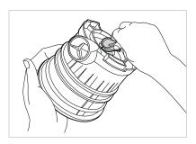
The silicone ring is removable for cleaning. After cleaning, place the silicone ring on as shown in the picture.
