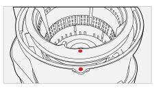
Place the juicing screw into the strainer.
