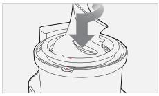
Note | The juicing screw needs to be locked in place in order to close the drum lid.
